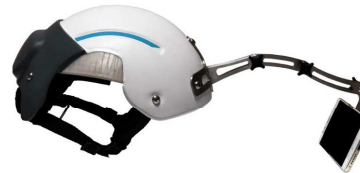
Fig. 6 : Final smartphone funduscopy device (lateral view)
